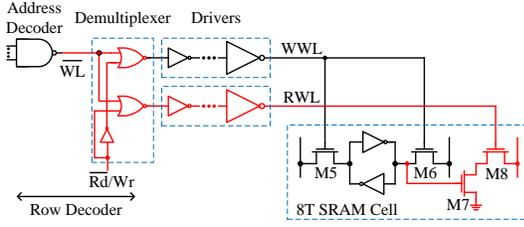
Fig. 7. Row decoder for an 8T SRAM cell. Highlighted parts with red color (demultiplexer, RWL drivers,  $M7$  and  $M8$  transistors) do not exist in conventional 6T cell designs.  $\overline{Rd}/Wr$  is 0 for read, and 1 for write operation.
