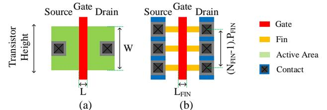
Fig. 6. Layouts of a transistor with channel width of  $W$  in (a) planar CMOS and (b) FinFET process technologies.
