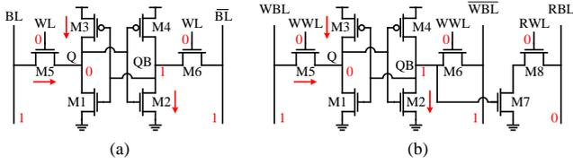
Fig. 2. Circuit schematics of (a) conventional 6T, and (b) 8T [2] SRAM cells.  $BL$  and  $WL$  denote bit-line and word-line, respectively. The 8T design contains separate  $BL$  and  $WL$ s for read and write operations. Arrows highlight subthreshold leakage paths in an idle SRAM cell (storing 0).
