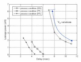
Figure 7. Power-delay curves for different levels of variability.
