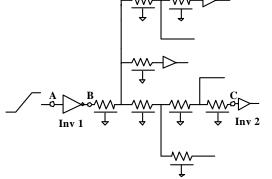
Figure 1: General delay model of interconnects which is driven by CMOS gates and driving another CMOS gates.
