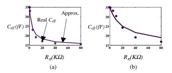
Figure 7: Effective capacitance for two different cases of  $T_{in}$  and driver sizes ( $C_1$ =15fF,  $C_2$ =20fF)(a) driver size=500 $\lambda$ ,  $T_R$ =100pS (b) driver size=100 $\lambda$ ,  $T_R$ = 200pS.
