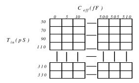
Figure 3: A two-dimensional delay table, one dimension is effective load and the other one is input transition time.
