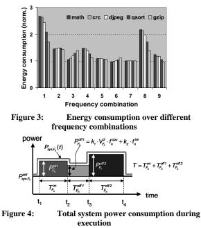
Energy consumption model in BitsyX is shown in Figure 4. Terms used in this figure are explained next.
