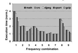
Figure 2: Execution time variation over different frequency combinations
