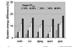
Figure 8: System energy difference: SE-DVFS vs. CE-DVFS
