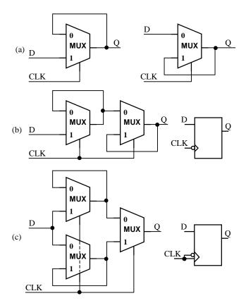
FIGURE 1 (a) Positive and negative level-sensitive latches; (b) SET flip-flop; (c) DET flip-flop
