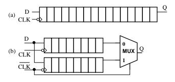
FIGURE 6. 2n-bit serial-in/serial-out shift register
