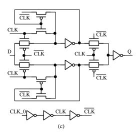
FIGURE 2 (a) The design of CMOS DET flip-flop in Ref.[7]; (b) A modified design of CMOS DET flip-flop; (c) The new design of CMOS DET flip-flop.
