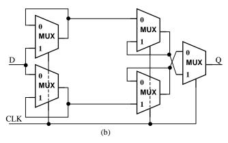
FIGURE 5 (a) Connection of two DET flip-flops in series; (b) Equivalent structure with SET flip-flops.
