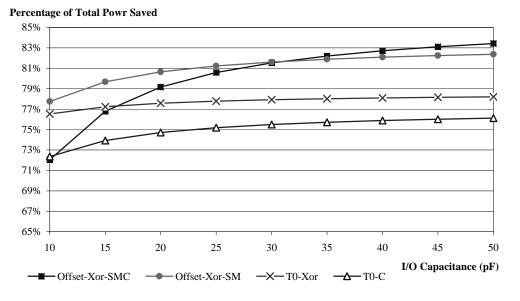
Figure 6- Comparison of total power savings for several encoding techniques.
