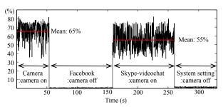
Fig. 15. The ratio of the power consumed by Camera digital to the power consumed by all the modules in Group 4.
