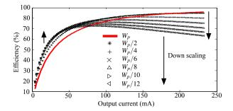
Fig. 9. Simulated power conversion efficiencies by changing the widths of the PMOS switch in Fig. 3.
