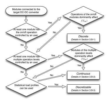
Fig. 10. Flowchart to classify  $f(I_{out})$  into three different cases.
