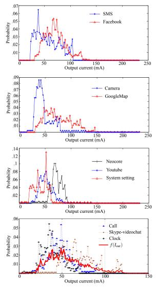
Fig. 5. Load current distributions of one core in MSM 8660 and a result of the derived  $f(I_{out})$ .
