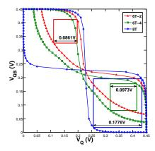
Fig. 3. Butterfly curves for 6T–2 ( $\triangle$ ), 6T–4 ( $\square$ ), and 8T( $\circ$ ) SRAM cells in 7nm FinFET. SNM values for each cell is included in the figure.
