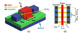
Fig. 1. FinFET device: (a) structure, (b) layout.
