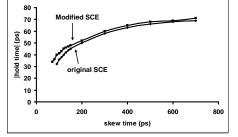
Figure 7. Effect of selective transistor sizing on hold time REFERENCES
