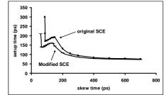
Figure 6. Effect of selective transistor sizing on setup time
