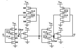
Figure 1. Schematic of a negative-edge triggered C<sup>2</sup>MOS FF.
